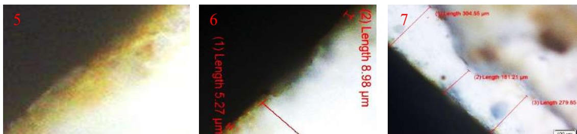
Figure 4: Photos (5-7) illustrate the cross-section investigation for the yellow pigment and the plaster to which the pigment was applied.
