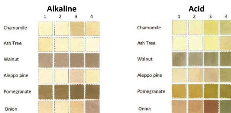
Figure 2: Cotton sample dyed in alkaline (pH 8) and acid (pH 4) medium (1-no mordanted sample; 2-sample treated with KAl(SO_4)_2 ; 3-sample treated with CuSO_4 ; 4-sample treated with FeSO_4 ).
